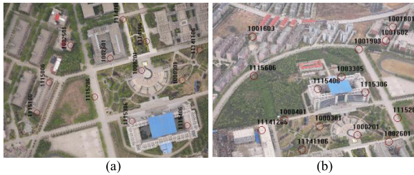
Fig. 8. Test images for real experiment. Red circles: control points. (The right-hand side image is rotated for better visualization.). (a) Central image. (b) Oblique image.
