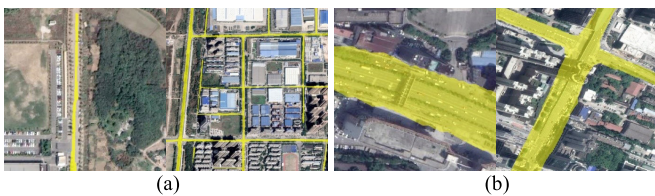
Fig. 6. (a) GPS trajectories raster is narrower than the road width. (b) GPS trajectories raster overflows road range.
