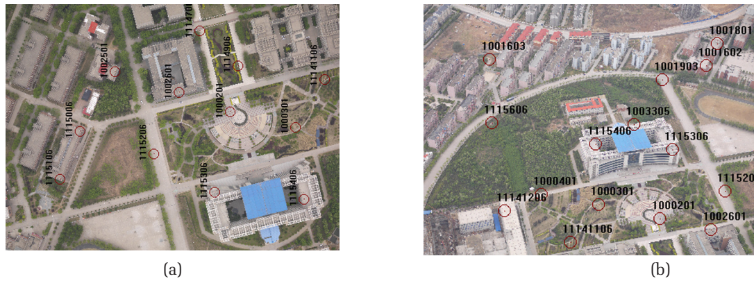
Figure 6. The aerial images used in this experiment. The red circles in the images are control points measured by GPS-RTK. (Figure 6a has been rotated for better visualization): (a) Image 1: captured by central camera of SWDC, and (b) Image 2: captured by an oblique camera of SWDC.
