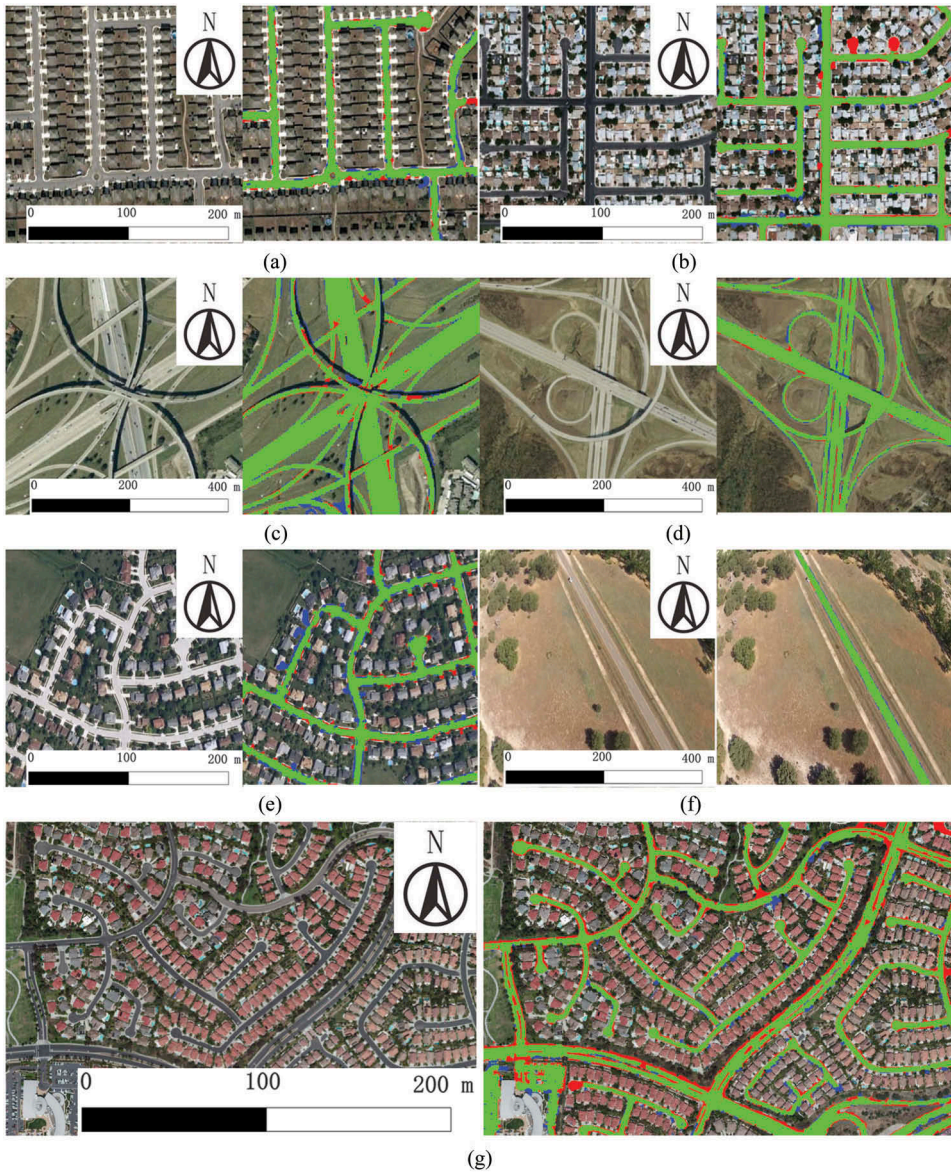
Figure 5. Road networks extracted in eight images of the Internet. Left images of (a)–(i): input images; right images of (a)–(i): our results. Green true positives, blue false positives, red false negatives.
