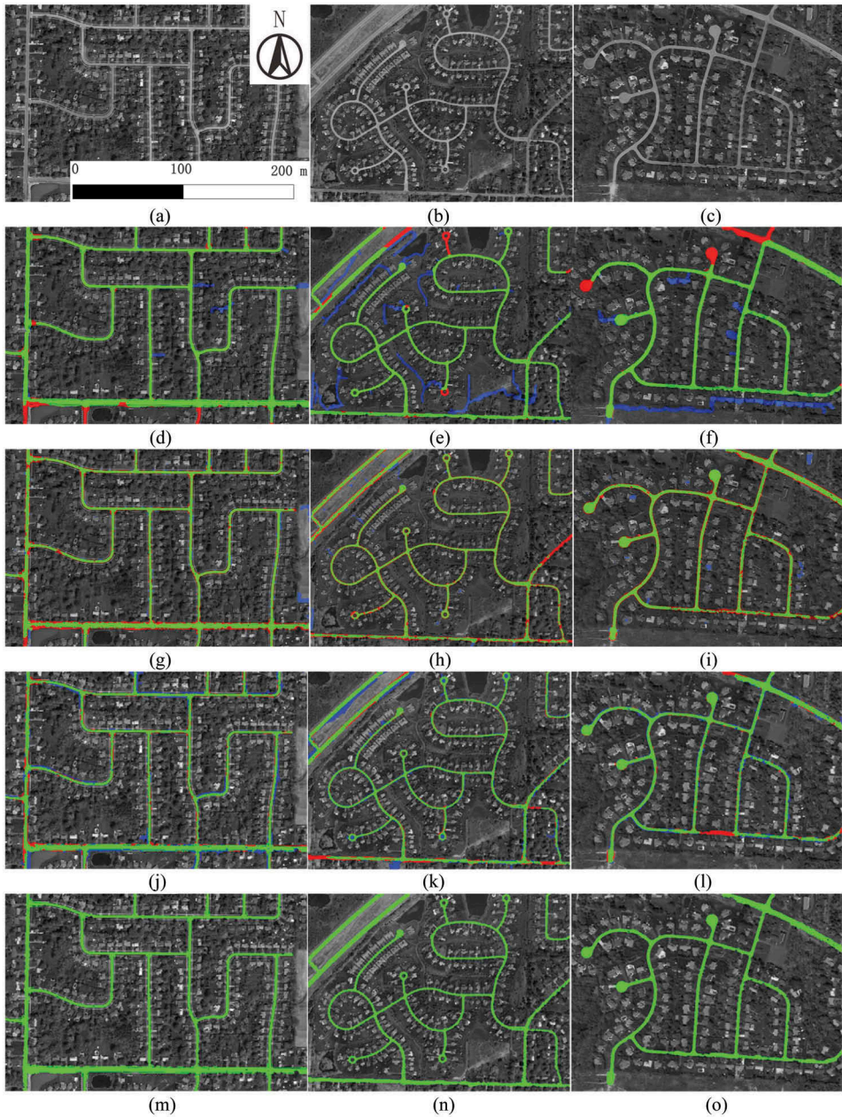
Figure 4. Road networks extracted in three patches of the EPFL. First row: original images; second row: Turetken's results; third row: Wegner's results; fourth row: our results; fifth row: ground truth. Green true positives, blue false positives, red false negatives.
