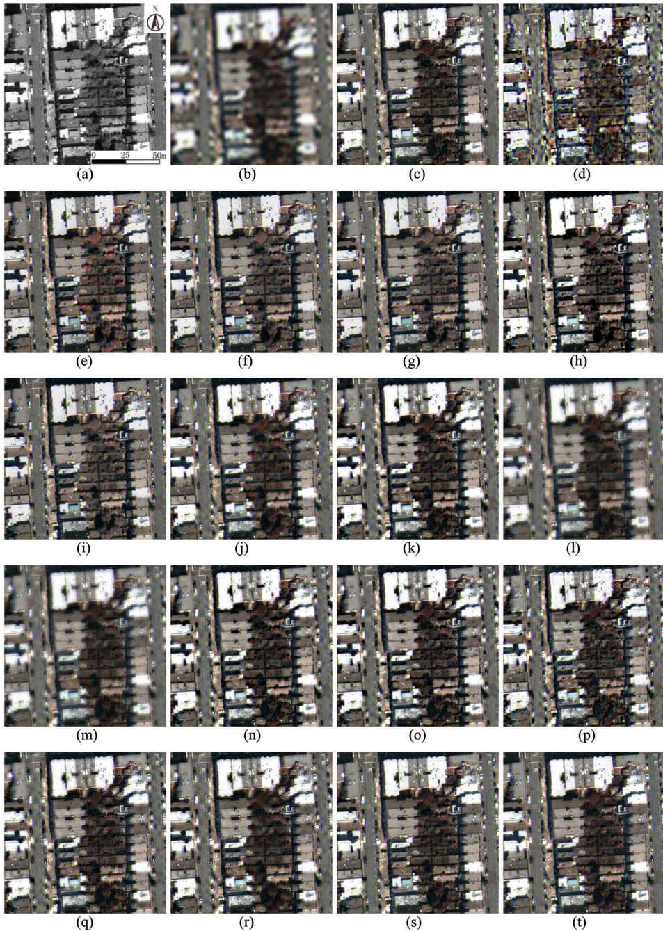
Figure 9. Pansharpening results for a sample image from the Worldview-2 data set. (a) Pan band. (b) Upscaled MS image. (c) Reference image. (d) BSDS. (e) Brovey. (f) GIHS. (g) GS. (h) GSA. (i) PCA. (j) PRACS. (k) ATWT. (l) ATWT-M2. (m) ATWT-M3. (n) AWLP. (o) HPF. (p) Indusion. (q) MTF-GLP. (r) SFIM. (s) Ours1. (t) Ours2.
